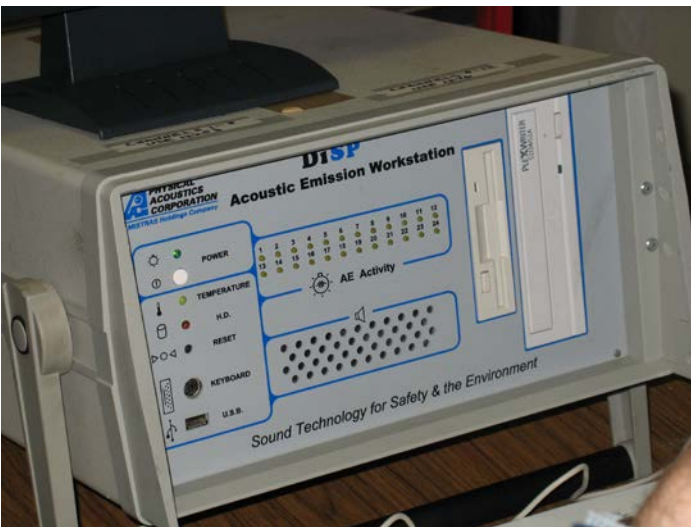
Figure 4. PAC DISP AE work station located in the cargo control room.
